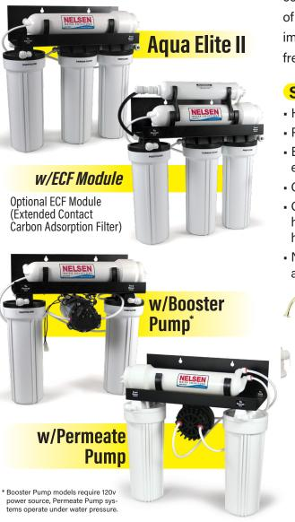
The **Aqua Elite Reverse Osmosis System** is simple to operate and requires no electricity\*. It works by forcing ordinary tap water (using household water pressure) through a semipermeable membrane which removes up to 99% of harmful water contaminants such as taste, odor, VOCs, fluoride, and toxic levels of arsenic, lead, nitrates, heavy metals & much more. These impurities are flushed down the drain leaving you with cleaner, fresher tasting water.
